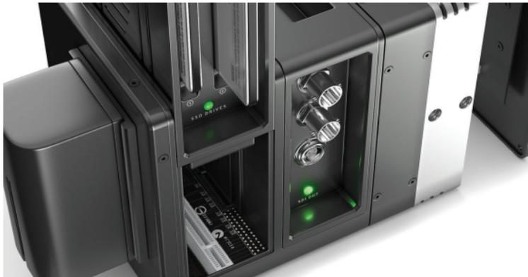
**AXIOM Gamma** is to become the very first entirely open and modular 4K Super 35 (sensor upgradeable) digital cinema production camera where every component can be replaced on demand to create a sustainable production camera platform and accompanying ecosystem (anyone can develop/sell new modules/accessories/services without any license/royalty restrictions). *Development until Q3 2016*
